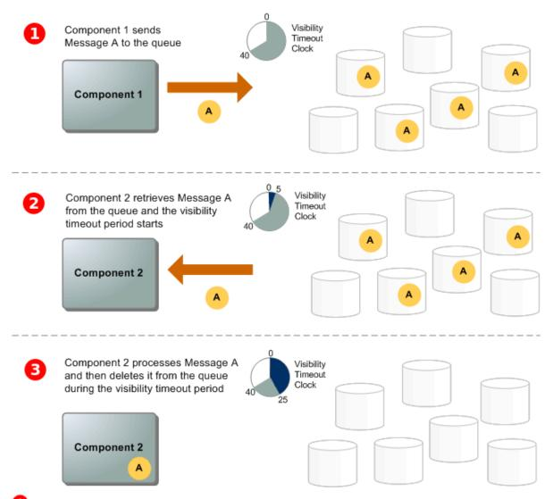
• A producer (component 1) **sends** message A to a queue, and the message is distributed across the Amazon SQS servers **redundantly**.
