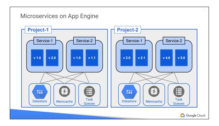
Services are a modular abstraction in App Engine; a way to break up the application into separate parts. Instead of architecting your entire application inside a single App Engine Service as shown on the previous slide, you can implement your application in multiple services. You can have more than one service in a project. You can also use multiple projects to further isolate services. Splitting traffic to different versions enables incremental rollouts and and A/B testing.
