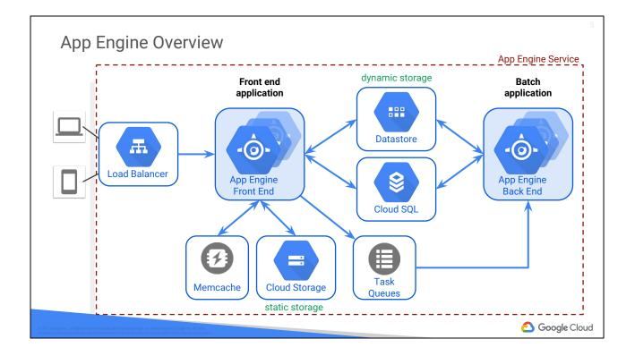
Front end is often critical to user experience (Load Balancer is built-in). Back end is for more intensive processing. This separation of function allows each part to scale as needed.
