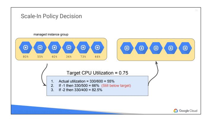
In this example, removing one VM doesn't get close enough to the target of 75%. Removing a second VM would exceed the target. Autoscaler behaves conservatively. So it will shut down one VM rather than two VMs. It would prefer underutilization over running out of resource when it is needed.
