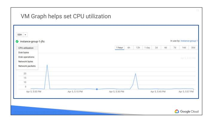
When you click on an instance group (or an individual VM) a graph is presented. The default display is CPU utilization. And you can look at the graph over different time frames. This is very handy for viewing actual traffic, looking for patterns, and determining how best to configure Autoscaling policy to meet changing demand.
