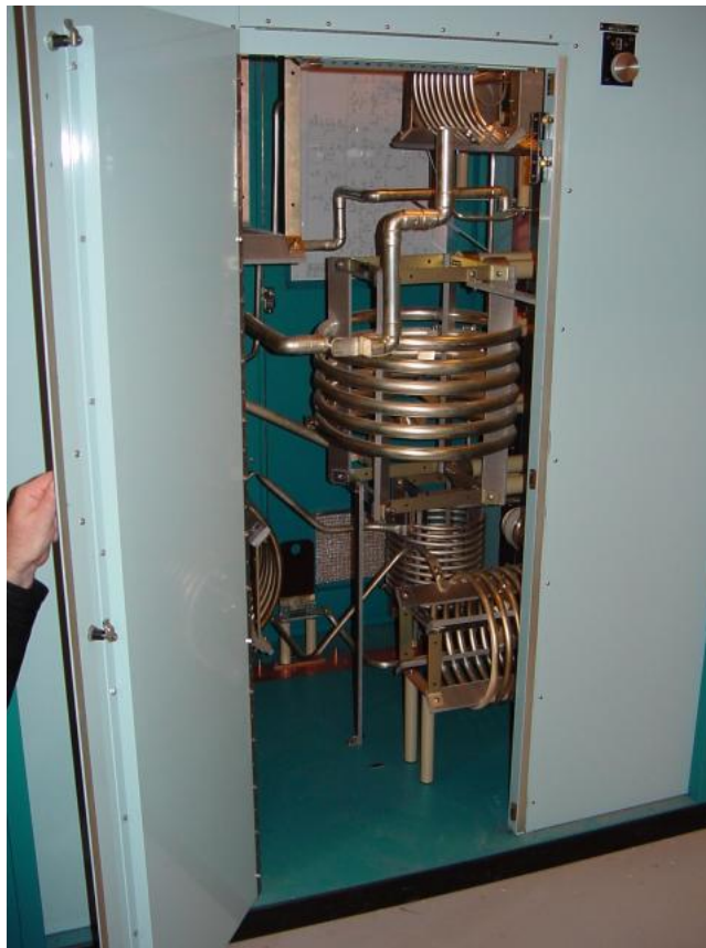
Figure 3.18: High power inductors formed from hollow tubes.
