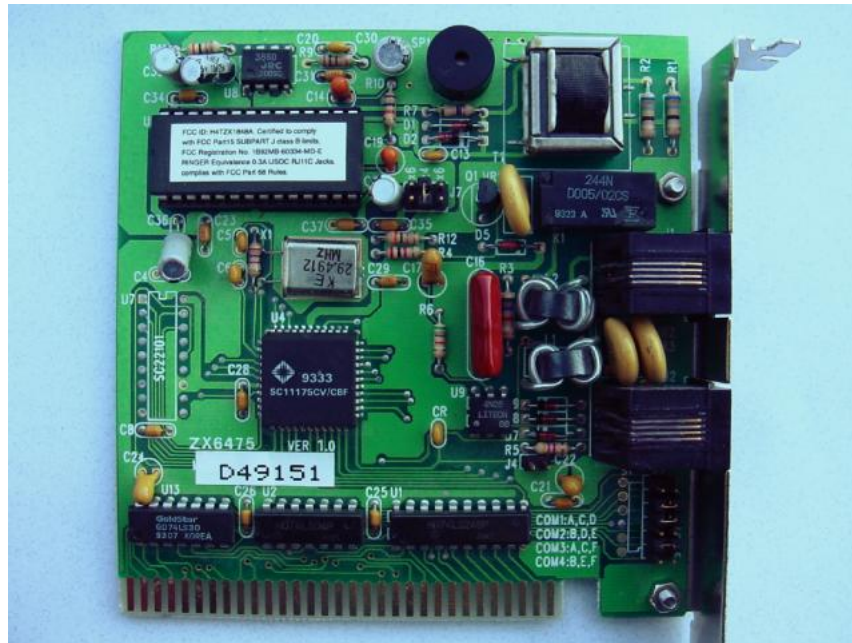
Figure 9.45: Printed circuit board mounted audio impedance matching transformer, top right.
