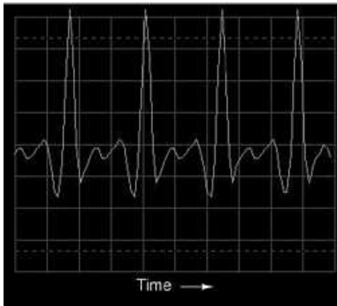
Figure 7.27: Oscilloscope display: waveshape of a trumpet tone.
