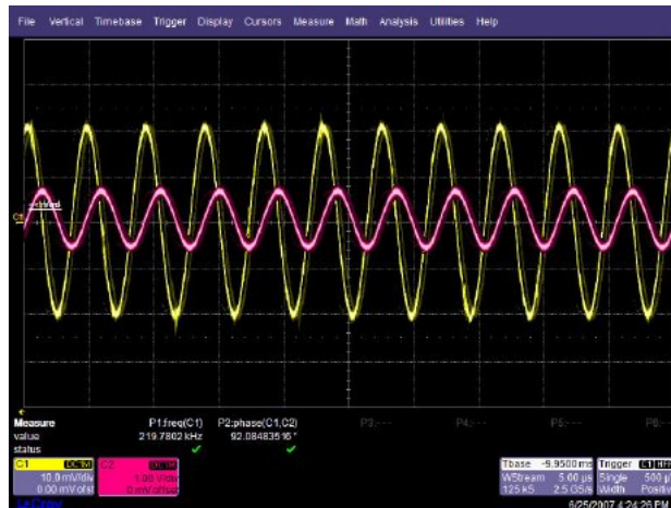
Figure 8.5: OPA227 A_v=50\text{dB} @ 220 kHz
