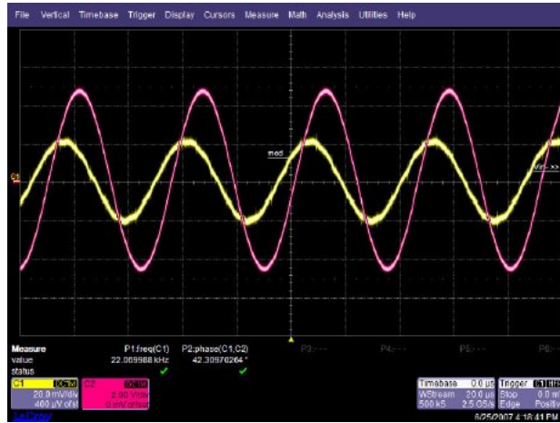
Figure 8.4: OPA227 A_v=50\text{dB} @ 22 kHz
