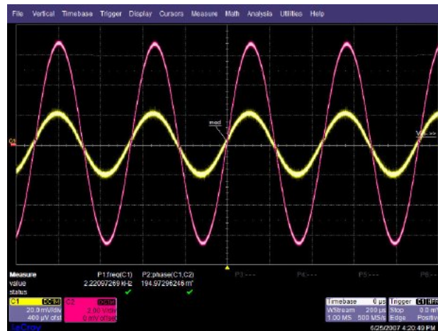
Figure 8.3: OPA227 A_v=50\text{dB} @ 2.2 kHz
