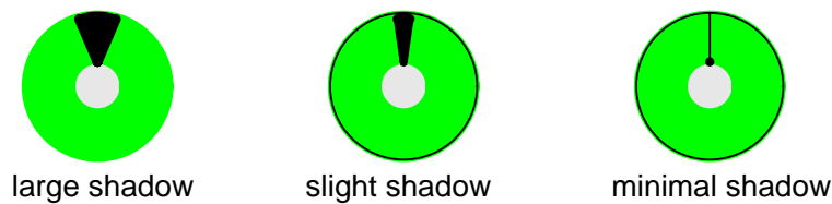
"Cat-Eye" indicator tube displays
