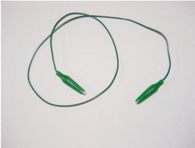
Jumper wires (home-made)
