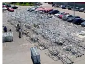
FM panel antenna for triangular mast assembled in-plant for factory test
