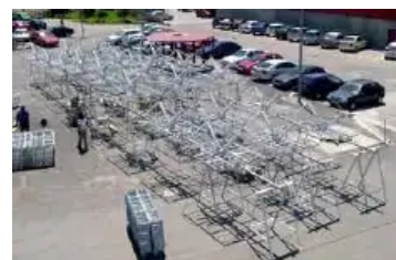
FM panel antenna for triangular mast assembled in-plant for factory tests
